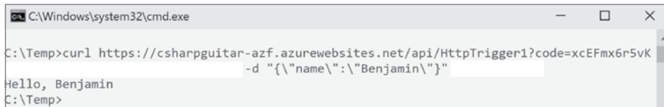
FIGURE 4.55 Consuming an HTTP-triggered Azure Function using curl
